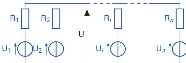
$$V = \frac{\frac{V_1}{R_1} + \frac{V_2}{R_2} + \dots + \frac{V_i}{R_i} + \dots + \frac{V_n}{R_n}}{\frac{1}{R_1} + \frac{1}{R_2} + \dots + \frac{1}{R_i} + \dots + \frac{1}{R_n}}$$
