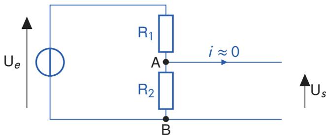
$$U_s = \frac{R_2}{R_1 + R_2} \cdot U_e$$
